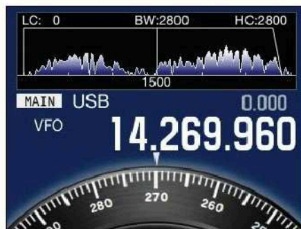
Figure 6 — This view of the smaller LCD panel shows operating frequency and mode, along with a graphic illustrating the filter bandwidth characteristics. The virtual analog dial skirt gives this thoroughly modern transceiver a retro touch from the classic TS-520S era of the 1970s. This image is a screen capture via the transceiver’s USB port.
