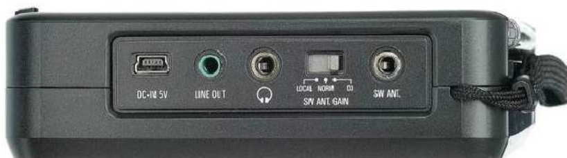
Figure 6 — The side panel of the Tecsun PL-880 has connections for headphones, LINE OUT, an external antenna and a USB port charging cable. The SW ANT GAIN switch selects among three sensitivity levels.
